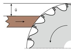
The recommended cutting speed is 70 – 90 m/sec. The upper value must be selected for diamond-tipped disk saw blades. A feed rate of 0,07 – 0,15 mm per tooth must be aimed at.
