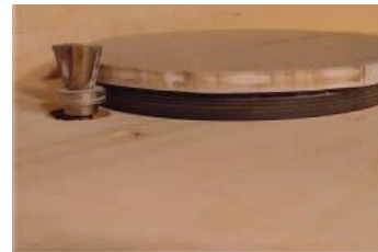
(6) Rout plug on router table
