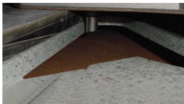
(3) Rout with 1/2" straight bit/1" guide
