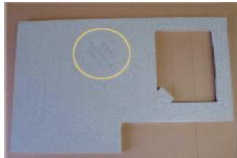
(1) Hot pot cracks
